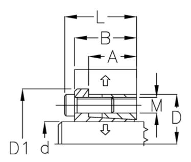
A mm = 25 B mm = 33 D1 mm = 88 d H8 mm = 42 D mm = 80 F kN torque = 72 L mm = 41 M mm = M8 P N/mm2 surface pressure on shaft/hub = 108T N m torque = 1509Ts N m bolt tightening torque = 41
